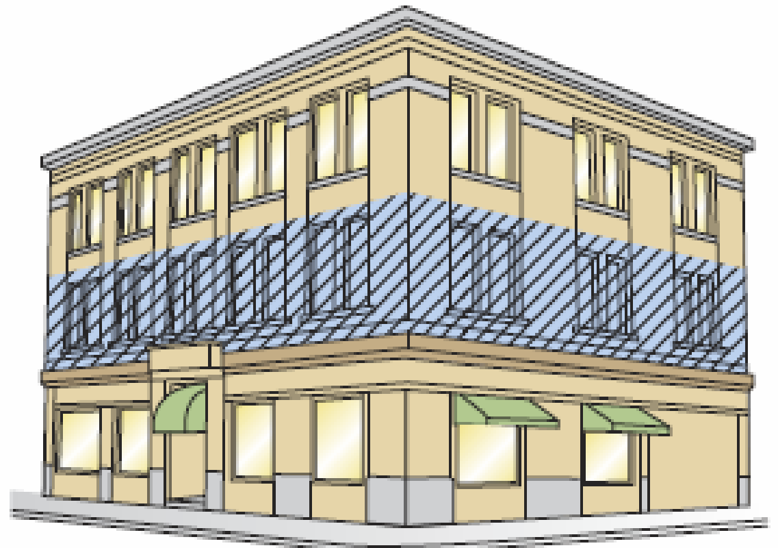
▨ Extent of required sprinklers
